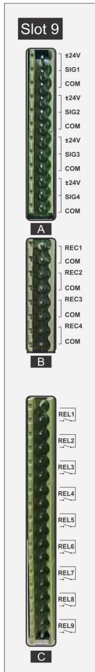
V6000/K is produced in two type: 2 input & 4 input versions. V6000/K rear panel has 12 terminals for connecting tachometers to it. There are three terminals per channel. First one ±24 is the power supply terminal for transducer it can be either +24 or -24 V DC based on the jumper selected.
